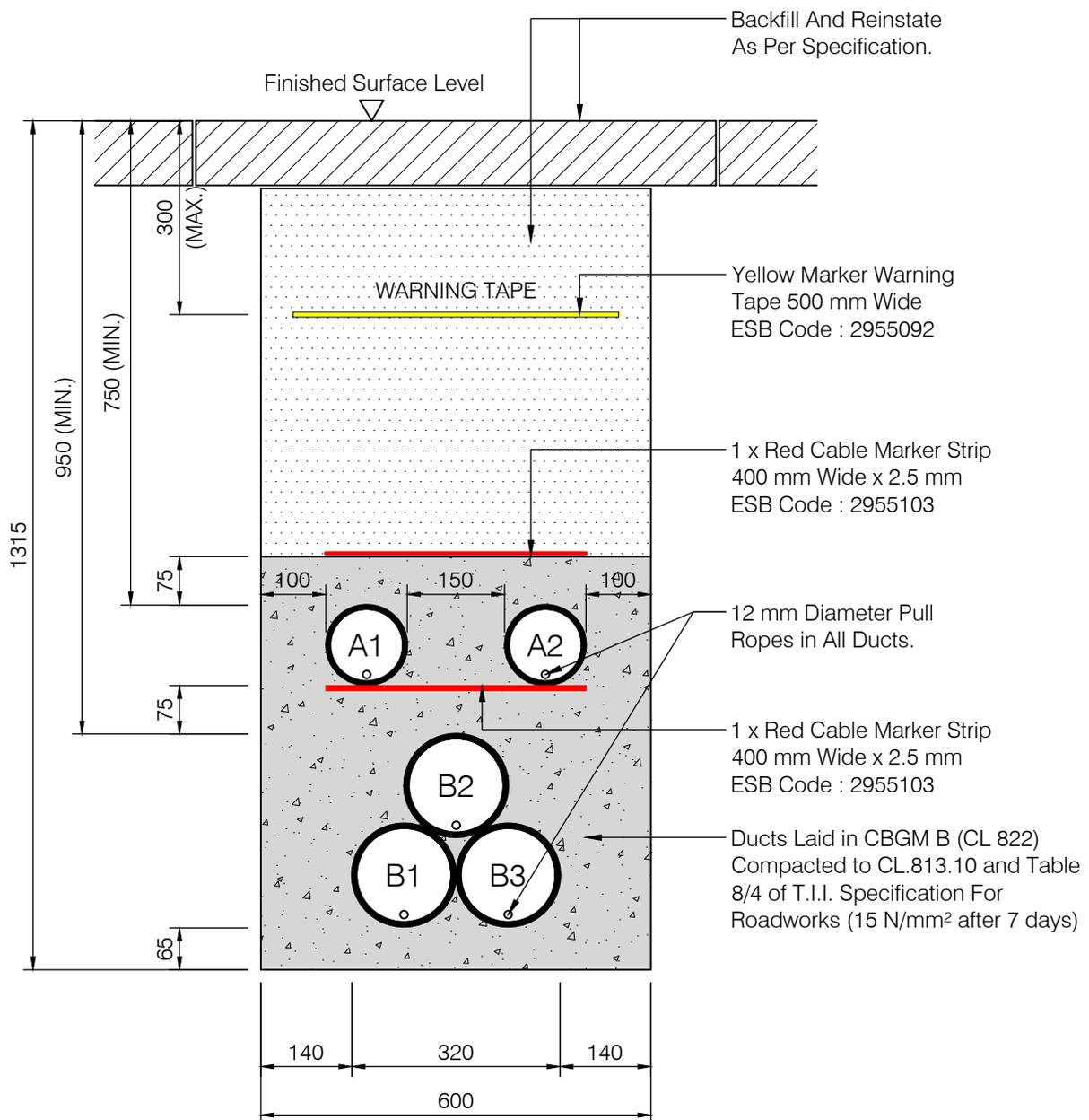
A=125 mm: Outer Diameter HDPE ESB Approved Duct, SDR=17.6
