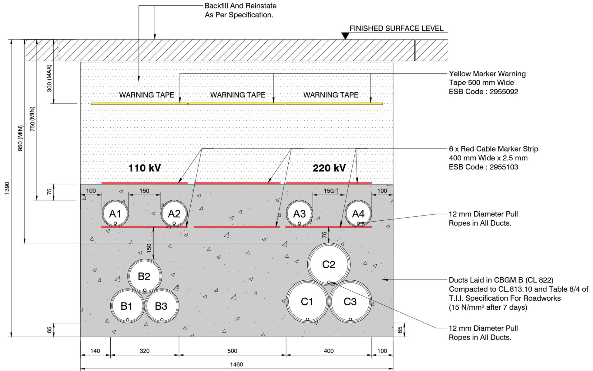
A = 125 mm: Ø OUTER DIAMETER HDPE ESB APPROVED DUCT, SDR = 17.6
